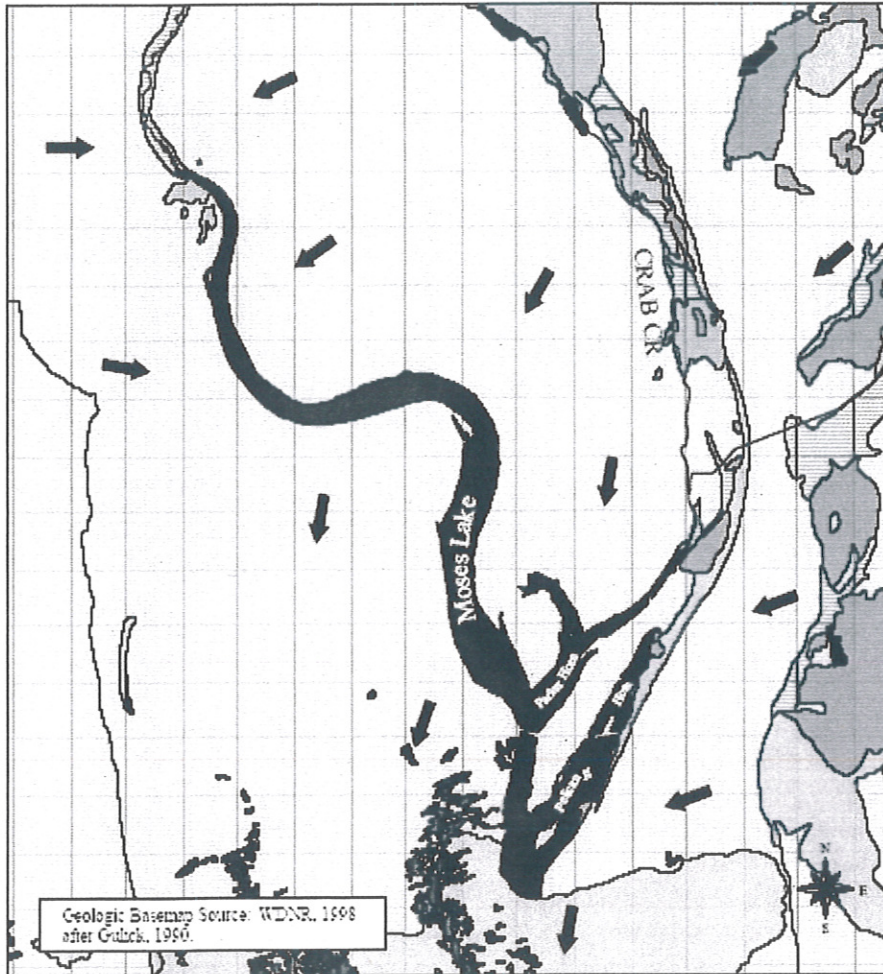
Figure 2. Groundwater flow direction in Moses Lake basin (arrows). Tan areas around lake are Pleistocene gravel and sand flood deposits (from Pitz 2003).
